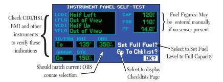
Once the database has been acknowledged, the *instrument panel self-test page* will appear. To ensure that your GNS 430 and any connected instruments are working properly, check for the following indications on your CDI/HSI, RMI, external annunciators and other connected instruments:
