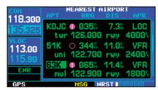
To scroll through the list, press the small right knob ( ), then rotate the large right knob ( ).
