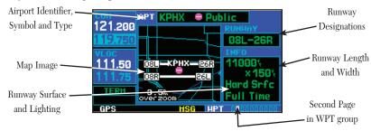
The airport runway page displays runway designations, length, surface type and lighting for the selected airport. A map image of the runway layout and surrounding area is also displayed on the airport runway page. The map image scale appears in the lower left corner and is adjustable using the key. For airports with multiple runways, information for each runway is available.
