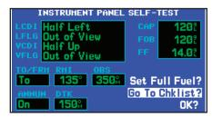
Select "Go To Chklist?" to display the checklist page and any available checklists. The GNS 430 can hold up to nine checklists with up to 30 entries in each checklist. The *instrument panel self-test page* includes selections to set fuel on board (FOB) to full capacity and access the *checklists page*. This allows you to quickly set fuel to full limits and display any checklists you've entered, such as start up or takeoff checklists.
