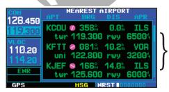
Whenever the GNS 430 is displaying a list of information that is too long for the display screen, a scroll bar will appear along the right-hand side of the display. The scroll bar graphically indicates the number of additional items available within the selected category.
