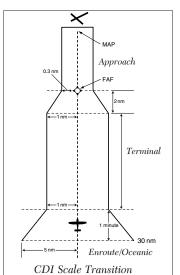
Unlike a VOR, the CDI scale used on GPS equipment is based on the cross-track distance to the desired course, not an angular relationship to the destination (see right). Therefore, the CDI deflection on the GPS will be constant regardless of the distance to the destination, and will not become less sensitive when you are further away from the destination. For more information on the CDI scale, see page 153.
