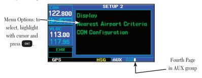
The *setup 2 page* provides access (via "menu options") to display adjustments, parameters which define the nearest airport search, and COM transceiver channel spacing. When a menu option is selected, the corresponding page will appear providing access to the various unit settings.
