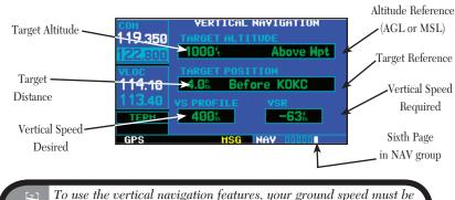
To use the vertical navigation features, your ground speed must be greater than 35 knots and you must be navigating to a direct-to destination or using a flight plan.
