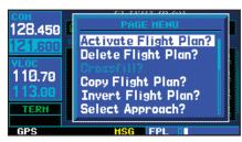
Select "Activate Flight Plan?" from the page menu to begin using the new flight plan.
