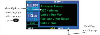
The *setup 1 page* provides access (via "menu options") to airspace alarms, CDI scale adjustment, an arrival alarm, units of measure settings, position formats, map datums and settings for local or UTC time display. When a menu option is selected, the corresponding page will appear providing access to the various unit settings.
