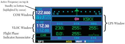
Pushing the small left knob ( ) activates the tuning cursor in the desired frequency window. To select the active frequency, you must first enter the frequency in the standby field, and use the ( ) key to move it to the active field.
