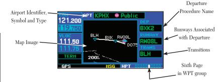
The *airport departure page* shows the available Airport Standard Instrument Departure (SID) procedures for the selected airport. Where multiple runways or transitions are associated with the departure procedure, that information may also be displayed. A map image provides a layout diagram for each departure, runway and transition.
