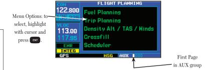
The *flight planning page* provides access (via "menu options") to E6B functions for fuel planning, trip planning, density altitude/true airspeed/winds aloft calculations and a "Crossfill" function to transfer flight plans/user waypoints to a second GNS 430. When a menu option is selected, the corresponding page will appear providing additional information and features.
