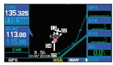
Once the standby frequency is selected, use the [] (flip-flop) key to make the frequency active for transmit and receive operations.
