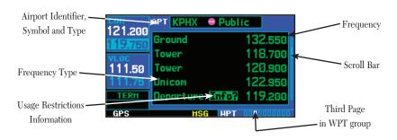
The *airport frequency page* displays radio frequencies and frequency types for the selected airport, as well as sector and altitude restrictions (where applicable). If the selected airport has a localizer-based approach, the localizer frequency(s) is also listed on the *airport frequency page*. The *airport frequency page* may be used to quickly select and tune a COM or VLOC frequency.
