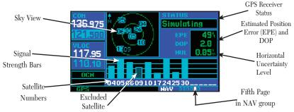
As the GPS receiver locks onto satellites, a signal strength bar will appear for each satellite in view, with the appropriate satellite number (01-32) underneath each bar. The progress of satellite acquisition is shown in three stages:
