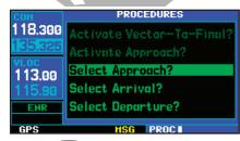
Press the ROO key to display the procedures page. Rotate the large right knob ( ) to select the desired option.
