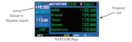
A frequency listed on the *NAVCOM page* can be quickly transferred to the standby field of the COM or VLOC windows. This time saving process prevents having to "rekey" a frequency already displayed elsewhere on the screen.
