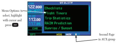
The *utility page* provides access (via "menu options") to checklists, a count down/up timer, trip timers, trip statistics, RAIM (Receiver Autonomous Integrity Monitoring) prediction, sunrise/sunset time calculations and software/database version information. When a menu option is selected, the corresponding page will appear providing additional information and features.
