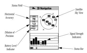
The GPSMAP 195's **satellite status page** provides a visual reference of satellite acquisition and receiver status, with a signal strength bar graph and a satellite sky view in the center of the page. The accuracy of your position reading is indicated on the upper left hand side of the page.
