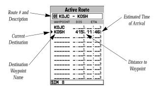
The last of the five main pages is the **active route page**. The active route page shows the GOTO waypoint or each waypoint of a route, with waypoint name, cumulative distance and ETA from your present position. The current destination waypoint is marked with an arrow on the left-hand side of the page. If no destination has been specified using the waypoint waypoints will be listed on the page.
