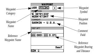
The last waypoint category available from the GPSMAP 195s were key is user waypoints. The user waypoint page allows entry of a desired waypoint by name/identifier and displays the waypoint's position, user comments and a reference waypoint field to calculate the distance and bearing from any other waypoint in the database. The user waypoint page can also be used to create up to 250 waypoints by manually entering a position or defining a range and bearing from an existing waypoint.
