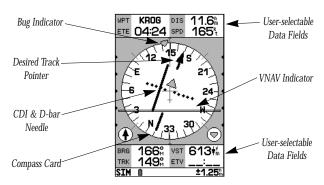
Whenever a GOTO, TracBack or route has been activated, the GPSMAP 195 will provide digital and graphic guidance to the destination waypoint with the **HSI page**. The top and bottom of the page features eight user-selectable **data fields** that display destination waypoint name (WPT), distance to waypoint (DIS), bearing to waypoint (BRG), estimated time enroute (ETE), ground speed (SPD) and more.
