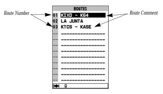
The second item on the main menu, 'Routes', provides another means of navigation over the direct GOTO. Unlike the GOTO function, which provides a course from present position to a single destination waypoint, the 'Routes' selection lets you create and store up to 20 reversible user-defined routes (numbered 0-19), with up to 30 waypoints in each route.
