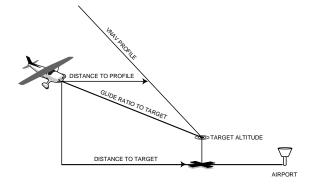
The **vertical navigation submenu** lets you create a VNAV profile which guides you from your present position and altitude to a final altitude at a specified location. Once the descent profile is defined, message alerts and additional data on the HSI page will keep you informed of your progress. To use the vertical navigation feature, your ground speed must be greater than 35 knots and you must be navigating using the GOTO feature or a route.
