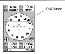
With the VNAV profile set, the HSI page will guide you through the maneuver. Data fields on the HSI page will indicate time to beginning of maneuver, time to target altitude and vertical speed to target. A VNAV indicator on the HSI display will guide you along the proper descent angle. Expect the following to occur when using the vertical navigation feature:
