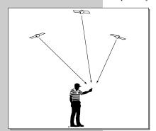
The GPSMAP 195's view of the sky will determine how fast you get a position fix, or if you get a fix at all. GPS signals do not pass through large obstructions made of wood or metal.
