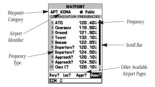
The airport communication page displays radio frequencies and their usage for the selected airport, and allows entry of a desired airport by identifier only (see page 28). The following frequencies are displayed if available:
