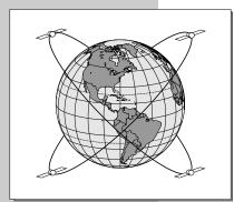
The 24 GPS satellites are constantly moving, orbiting the earth twice a day. In order to calculate your position, the GPS receiver needs to continuously "see" at least three satellites.
