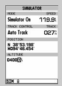
The simulator submenu allows you to enable/disable simulator mode, define a starting position/altitude, and define an initial ground track and speed.
