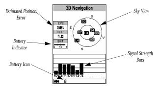
The GPSMAP 195's **status page** provides a visual reference of various receiver functions, including current satellite coverage, receiver operating mode, battery strength and current receiver accuracy. The status information will give you an idea of what the receiver is doing at any given moment.
